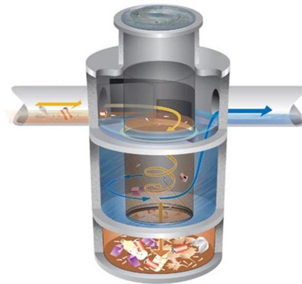
**Figure B-3: Gross Pollutant Trap Schematic<sup>9</sup>**
